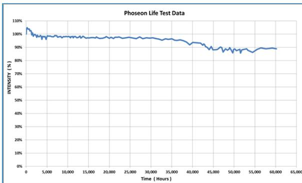
Phoseon's extensive reliability testing includes highly accelerated life testing, temperature, and vibration assessments to ensure products are rugged and reliable in even the harshest environments. The light sources are stressed with decreased air flow, high temperatures and other parameters that mimic the harsh working conditions of industrial LED curing equipment.
