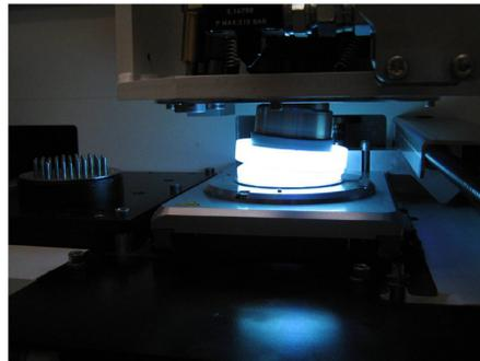
Satisloh's On-Block Technology with Phoseon's UV LED Curing Lamp
