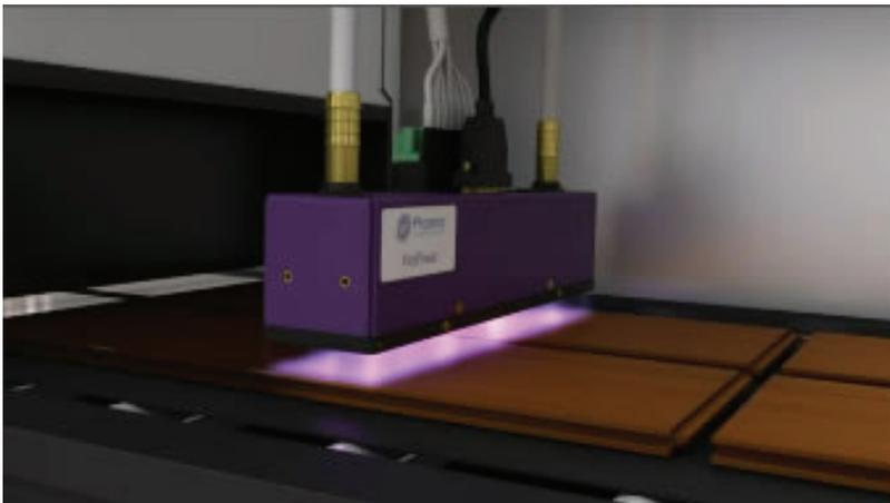
UV LED curing solutions are being utilized in the wood coating industry because they offer highly reliable UV curing due to being a solid-state device. They provide deep through-cure in course-grain woods and allow low surface temperatures that enable cheaper raw inputs.
